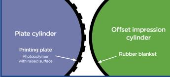
Raised portions of the printing plate transfer the ink to a rubber blanket on the offset cylinder.
