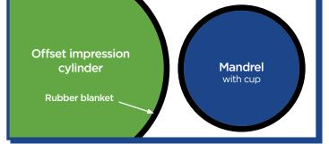
The image on the rubber blanket, consisting of all combined colors, is transferred (i.e. offset) in one pass onto the plastic container.
