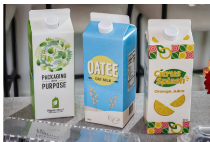
Paper forming: gable top beverage cartons
